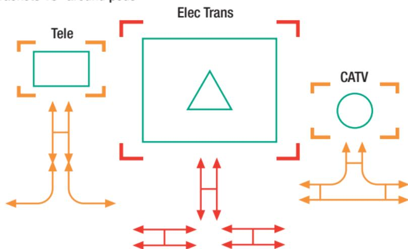
Markings start outside of brackets. Dig by hand inside the marked area.
