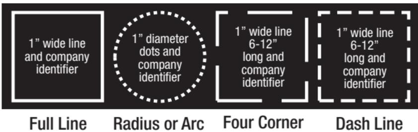
Premark the proposed area of excavation by using: a continuous line, dots marking a radius or arc, dashes marking the four corners of a project, or dashes outlining the excavation project. Make the dash about 6" to 12" in length and 1" in width. Space them between 4' to 50' apart. Make the marks close together enough to be seen by utility locators. Dots of about 1" in diameter are typically used to define arcs or radii and can be placed at closer intervals instead of the dashes.
